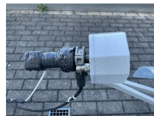
DualFeed Patch from PA3FYM, LNB: GooBay 67269 modified for 25 MHz Ref. over the coax, and 1.2m Offset Dish
