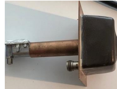
Modified LNB 0.2 PPM with POTY Antenna by DG9BFC
