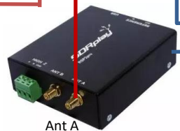
SDRPlay SDR Receiver RSP2Pro (as panadapter for IC-9700)
