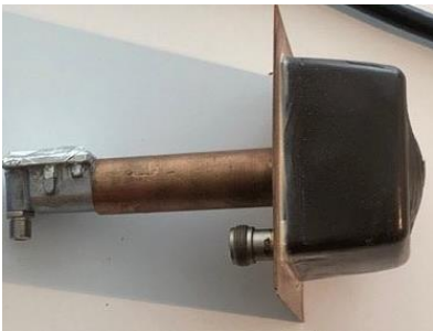
Modified LNB 0.2 PPM with POTY Antenna
