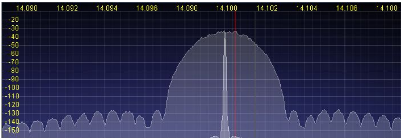
Figure 110: 25 Hz CWL Filter at 192 kHz Sample Rate/256 Buffer Size (Wide) and 48 kHz/4096 (Narrow)
